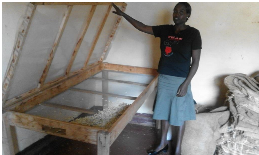
Solar drier for pyrethrum flowers for smallholders - demo
